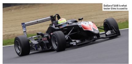
Dallara/F308/2008 CHASSIS: Carbon and honeycomb composite monocoque DESIGNER Ferdinando Concari ENGINE: HWA Mercedes-Benz 4-cylinder, 16-valve and double-overhead camshaft 1997cc POWER OUTPUT: 207bhp (26mm air restrictor) GEARBOX: Hewland FTR200, 6speed, sequential shift
