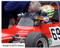
MAKE/MODEL/YEAR: LOTUS/69/1971 CHASSIS: Tubular steel, alloy nanelled DESIGNER: David Baldwin ENGINE: Lotus LF 4-cylinder twin-cam 1594cc **POWER OUTPUT:** 125bhp (21.5mm air restrictor) GEARBOX: Hewland Mk8,
