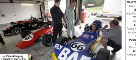
MAKE/MODEL/YEAR: MARCH/743/1974 CHASSIS: inium monocoau DESIGNER: Robin Herd ENGINE: yota Novamotor 2TG 4-cylinder twin-cam 1998rr **POWER OUTPUT:** 165bhp (24mm air restrictor) GEARBOX: ewland Mk9, 5-speed Monaco, there was an international victory at Hockenheim.
